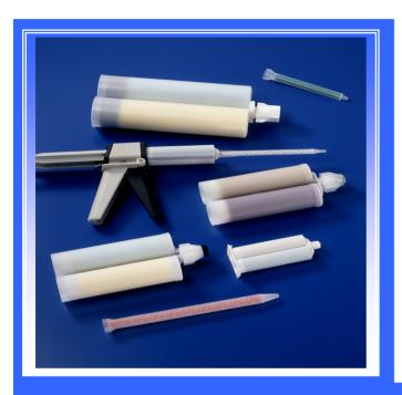
These systems are designed primarily for 1:1, 2:1, 4:1, and 10:1 parts-by-volume ratios. Total capacities can range from 50ml to 1500ml. Cartridge maybe used at different times while only replacing the static mixer nozzle.
