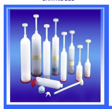
The "barrier" cartridge has a foiled mixer dasher that is held in place inside the cartridge with a cinch tape on the outside of the cartridge. The foil separates the resin and curative. This cartridge is typically used with systems that are between 1:1 and 10:1 parts-by-volume ratio.
