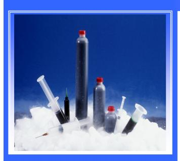
This procedures involves mixing Part A and Part B of a material at the specified ratio to a homogeneous blend, then degassing or centrifuging before filling the customers chosen container and immediately subjecting the package to an approximate 90 – 100 degrees below zero Fahrenheit. This immediately suspends any chemical reaction needed for material cure. Frozen containers are packed in dry ice and shipped overnight.
