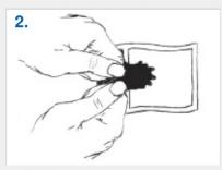
Apply thumb pressure to rupture burst seal.
