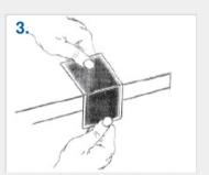
Mix thoroughly on table edge or any 90 degree surface until well mixed.
